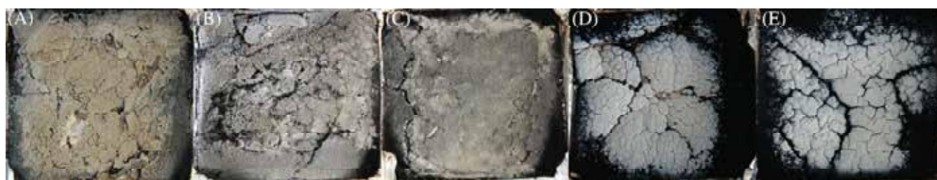
FIGURE 10 Digital photographs of the wood-polymer composites (WPCs) residuals: unfilled WPCs, A; micron-SiO 2 filled WPCs via dry dispersion, B; micron-SiO 2 filled WPCs via wet dispersion, C; nano-SiO 2 filled WPCs via dry dispersion, D; nano-SiO 2 filled WPCs via wet dispersion, E [Color figure can be viewed at wileyonlinelibrary.com ]
