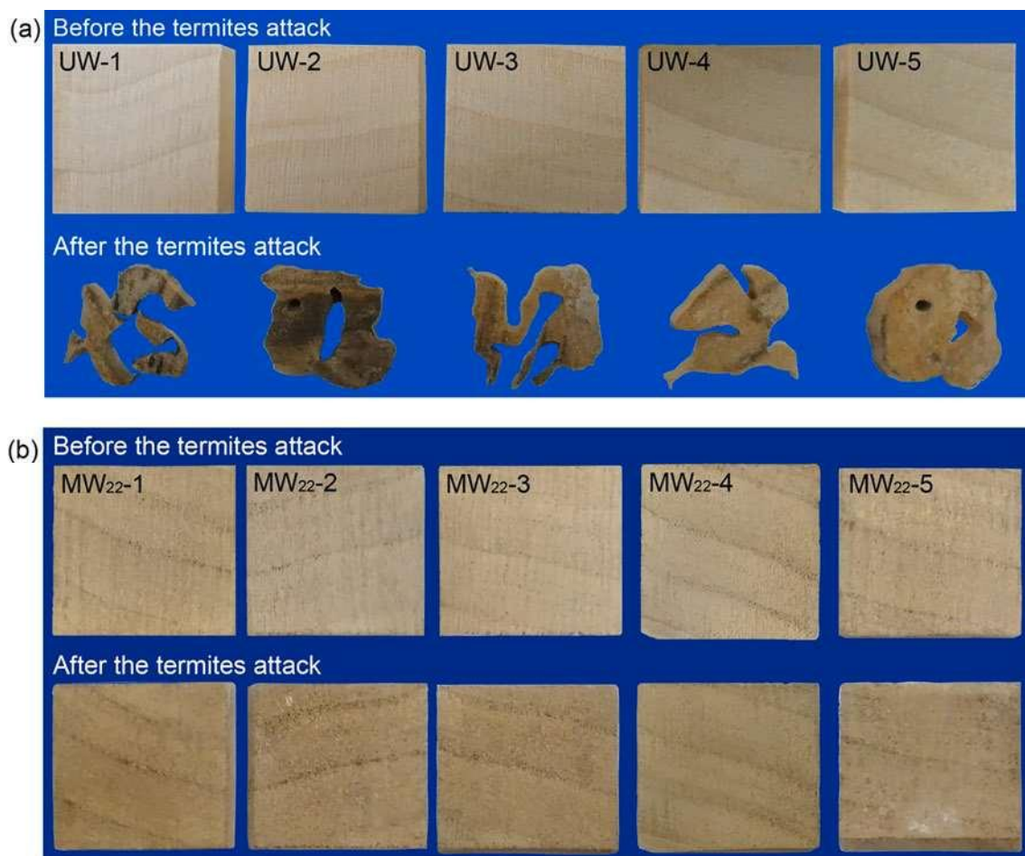
Fig. 16. Appearance of (a) untreated wood (UW) and (b) mineralized wood with 22.1% ZnB (MW 22 ) before and after termite attack.
