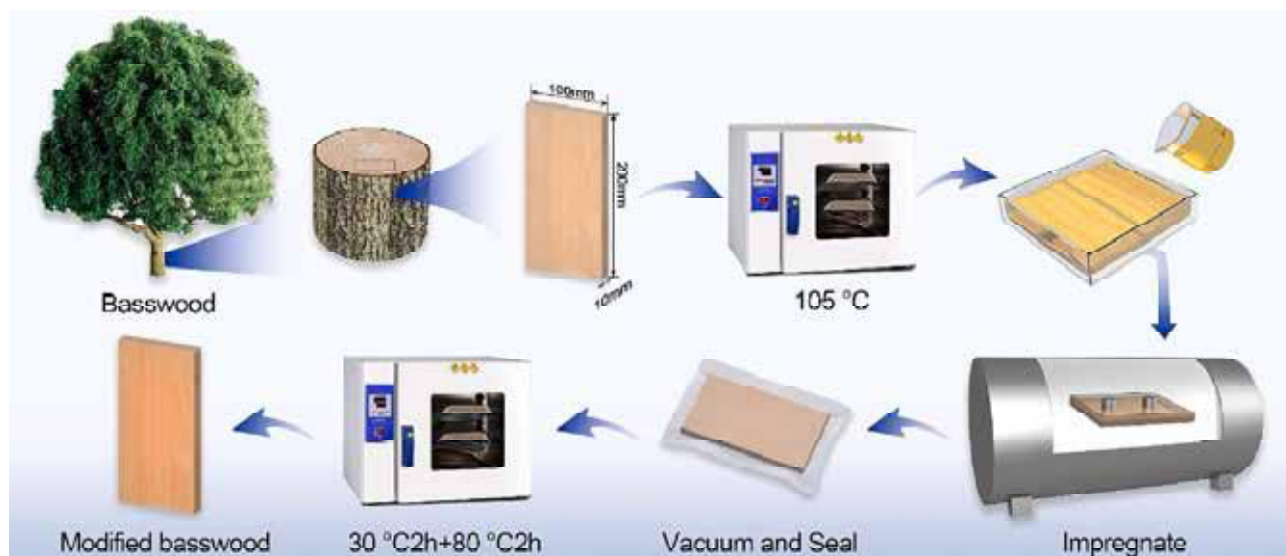
Fig. 1. Schematic diagram of the preparation of modified basswood.
