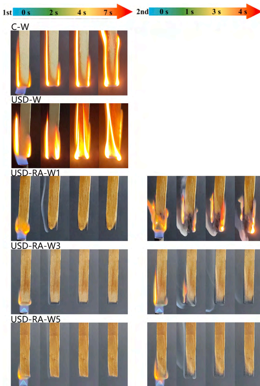
Fig. 10. Digital photos of C-W, USD-W, and USD-RA-W during UL-94 test.
